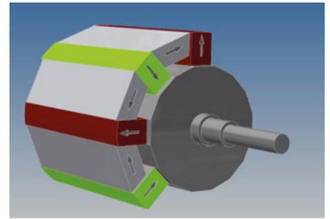
**Magnetic drum separator neodymium power supply, high intensity**
