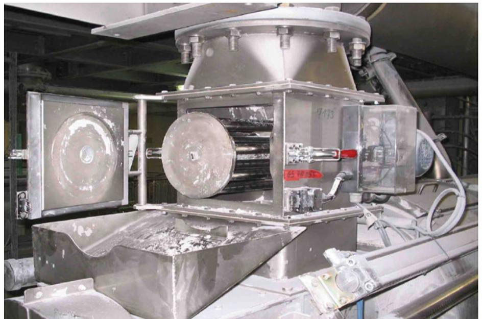
advantages: the magnetic field strength at the pipe is considerably higher. This is important for capturing 316 stainless steel particles. Moreover, no product comes between the magnetic bar and the extractor tube.
