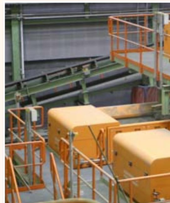
*Three non-ferrous separators type NF1500 on plateau in combustion slag reprocessing*
