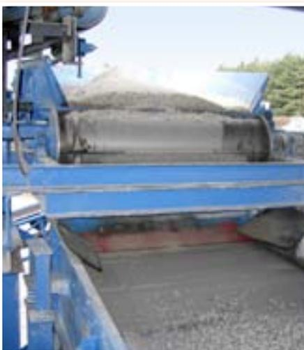
NEOFLUX® drum magnet for glass recycling
