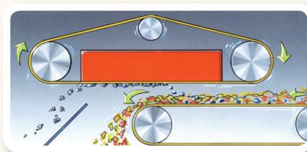
Permanent and electromagnetic overbelt magnets.
