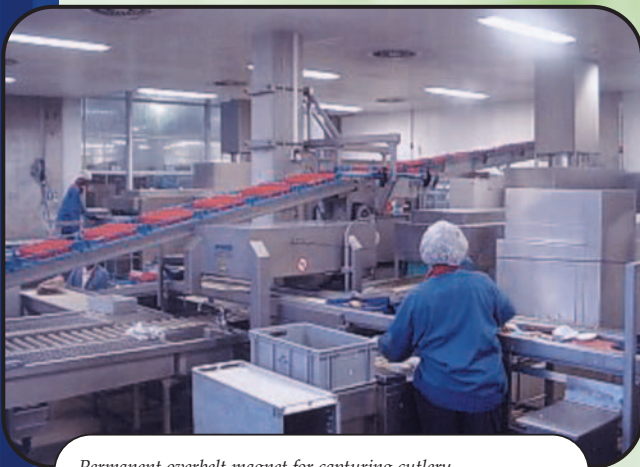
Permanent overbelt magnet for capturing cutlery.
