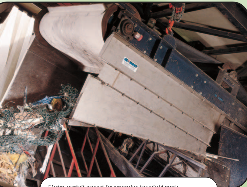
Electro overbelt magnet for processing household waste.
