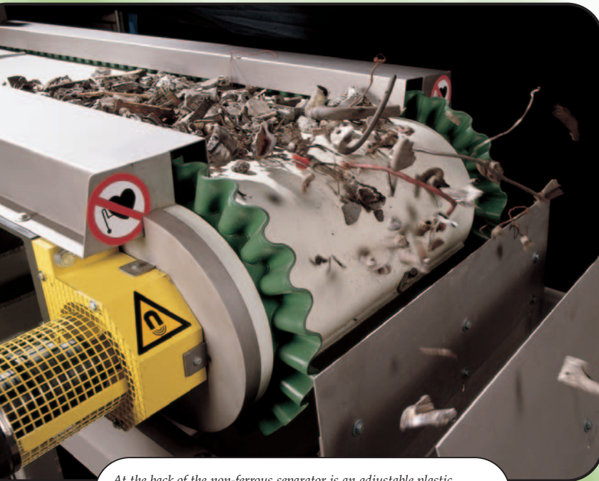
At the back of the non-ferrous separator is an adjustable plastic separation plate for optimal results.
