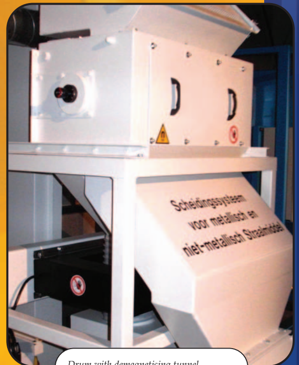
Drum with demagnetising tunnel.
