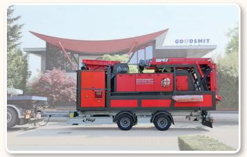
The mobile "next generation" Eddy Current separators can be used with both fine and normal fractions - even with small quantities - and placed in different locations.
