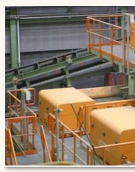
Three non-ferrous separators type NF1500 on plateau in combustion slag reprocessing
