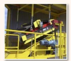
Electro overbelt magnet for the wood processing industry
