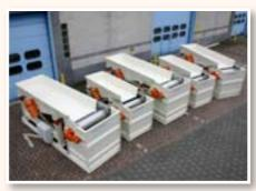
NEOFLUX® drum magnets with vibrating chute
