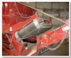
NEOFLUX® overbelt magnet on wood shredder (lightweight and compact)
