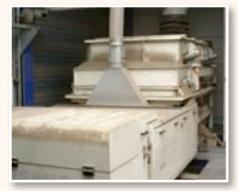
Non-ferrous separator for biofuel (for green electricity)
