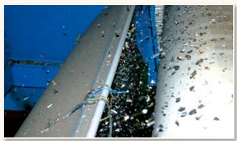
Detail of non-ferrous separator (width: 1500 mm) for WEEE scrap
