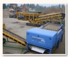
Non-ferrous separator with a width of 2000 mm for processing of waste wood
