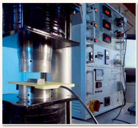
A Permagraph determines the magnetic energy
