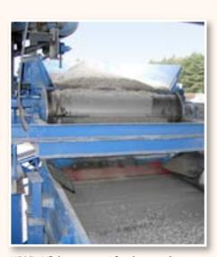
NEOFLUX® drum magnet for glass recycling
