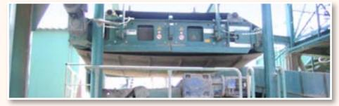
2 meter wide electro overbelt magnet for processing construction and demolition waste
