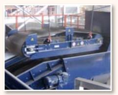
Permanent overbelt magnet in line above conveyor belt
