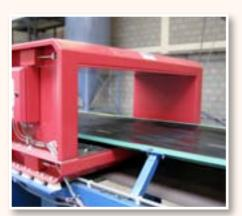
Mounting of metal detector. Clearly visible: metal-free zone
