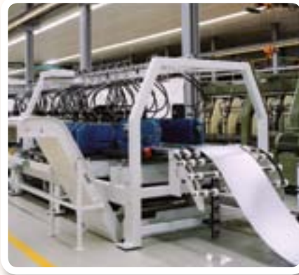
Slide bed conveyor mounted under a stamping machine to carry off the pressing scrap.
