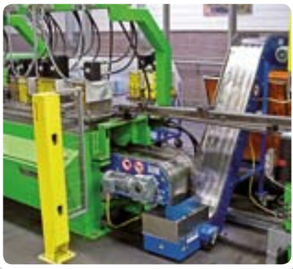
Combination flat bed & swan neck conveyor for discharge of punched parts.
