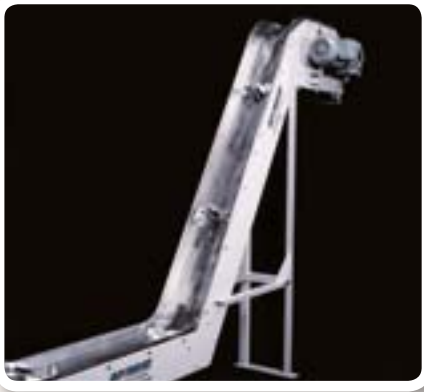
Slide bed conveyor mounted under a stamping machine to carry off the pressing scrap.
