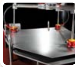
The MagVacu gripper contains double power (magnet and vacuum) and with this double safety, especially suitable for handling of non-ferrous parts of perforated in p.e. the automotive industry.
