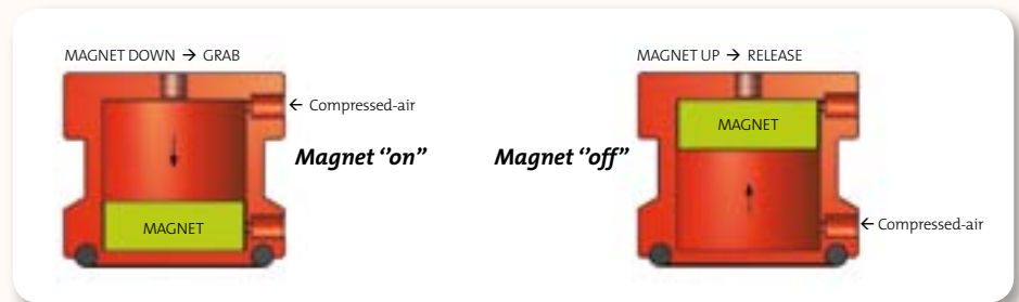
Magnet gripper with flexolink spring plunger for angle compensation of appr. 5°.
