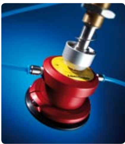
Vacuum suction pad at the bottom of the gripper, for the lifting of non-magnetic parts. Plunger with flexolink for more variation in the engagement moment, so that the gripper can also firmly grasp the object under an angle.
