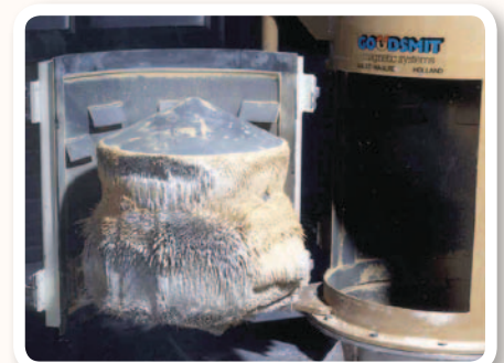
A pipe magnet removes very fine Fe particles in the ceramic industry.
