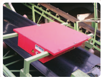
Ferrite plate magnet above belt, for removal of fe-particles from potting soil.
