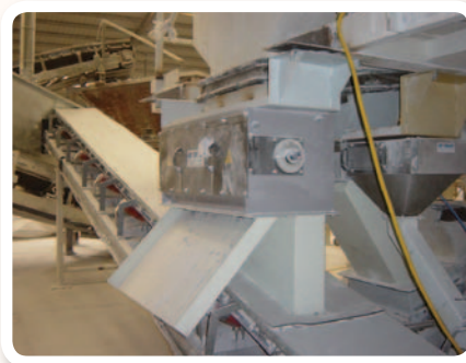
Drum magnet with axial pole of 3000 Gauss is suitable for applications such as those found in the ceramic industry.
