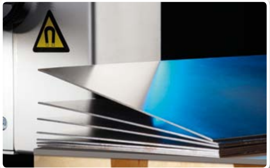
Switchable pneumatic operated sheet separator.
